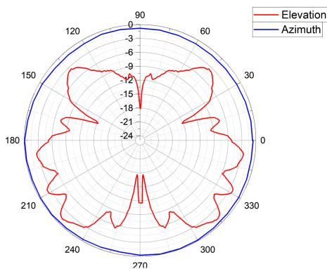
Frequency: 5.15 GHz Max Gain: 5dBi
